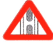
Gap in Median
